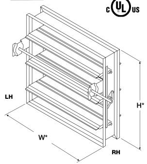
\*W&H dimensions furnished approximately <sup>1</sup>/4 in. (6 mm) undersize. (Add sleeve thickness for overall sleeved damper dimension) Right hand drive is shown. Left hand drive is available upon request.
